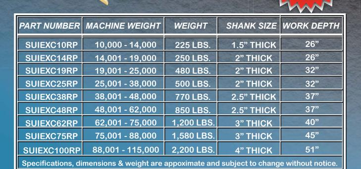
Steel Unlimited, Inc. ripper shanks are made of tough abrasion resistant alloy steel and hardened for strength and maximum wear life. Custom ripper shanks are available, including weld on noses, ripper teeth and shank protectors to suit any ripping application or machine size.
